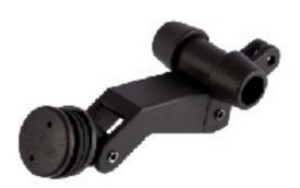
This easy to operate window hold-open is designed to fit comfortably using a two finger operation for top and side hinged venting windows for on and off-highway vehicles. It features an over center design that orientates the window at fully closed and fully open positions and an optional quick release pin in bright red nylon or steel.
